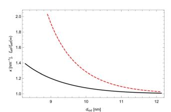
Fig. 10 The electrostatic screening length and effective filament charge within colloidal membranes. The inverse Debye length,  $\kappa$  (black line), and the corresponding dimensionless effective linear charge density  $\xi_{\rm eff}$  (dashed red line) are plotted as a function of inter-rod separation. The effective charge density is normalized by its bulk value,  $\xi_{\rm eff}$  = 36.15 for  $\kappa_{\rm D}$  = 1 nm<sup>-1</sup>.
