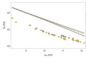
Fig. 11 The theoretical predictions for the osmotic pressure as a function of inter-rod separation are shown for persistence lengths corresponding to fd-wt ( $l_p = 2~\mu m$ , blue line) and fd-Y121M ( $l_p = 10~\mu m$ , orange line), overlaid on the experimental data. The theoretical results are obtained from eqn (4)–(9). The dashed black line shows the result in the rigid rod limit ( $l_p = \infty$ ).
