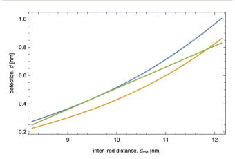
Fig. 13 The scale of filament undulations, d, calculated from eqn (4) is shown for fd-wt (blue line) and fd-Y121M (orange line) as a function of inter-rod separation. The straight line is an effective Lindemann criteria,  $d = 0.17(d_{rod} - \sigma)$ , which estimates the inter-rod separation at which the membrane melts for each case
