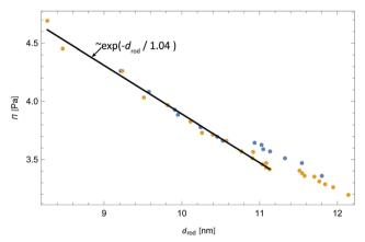
Fig. 12 Osmotic pressure of crystalline membranes scales exponentially with filament separation. The experimentally measured equation of state for fd-wt and fd-Y121M is plotted as a function of the inter-rod separation. The log scale Y-axis illustrates the exponential decay. The solid black line is a best fit to the data within the crystalline regime, yielding a decay length of  $\kappa_{\rm eff}^{-1}=1.04$  nm.
